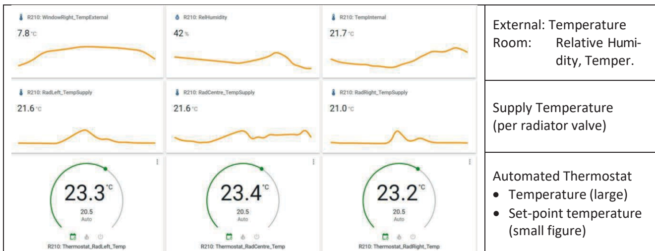
Figure 5: Initial screenshot from the BAC-system's monitoring dashboard
