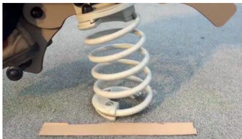
Figure 10: Students measuring the deflection of the spring
